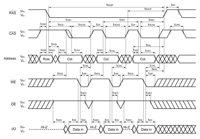
**Remark** In the hyper page mode (EDO), read, write and read modify write cycles are available for each of the consecutive  $\overline{CAS}$  cycles within the same  $\overline{RAS}$  cycle.
