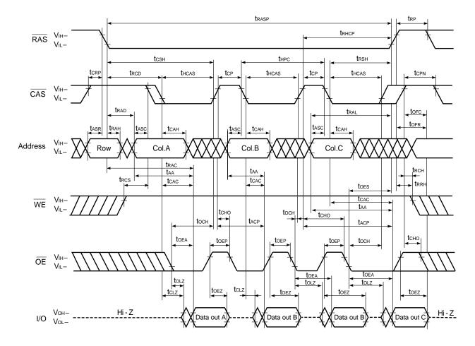
**Remark** In the hyper page mode (EDO), read, write and read modify write cycles are available for each of the consecutive  $\overline{CAS}$  cycles within the same  $\overline{RAS}$  cycle.
