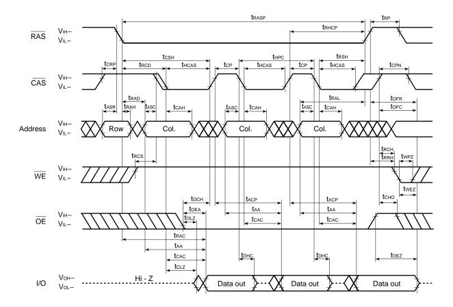
**Remark** In the hyper page mode (EDO), read, write and read modify write cycles are available for each of the consecutive  $\overline{CAS}$  cycles within the same  $\overline{RAS}$  cycle.
