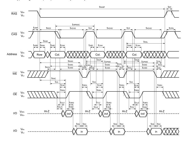
**Remark** In the hyper page mode (EDO), read, write and read modify write cycles are available for each of the consecutive  $\overline{\text{CAS}}$  cycles within the same  $\overline{\text{RAS}}$  cycle.
