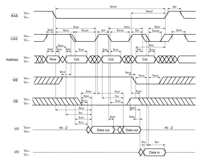
**Remark** In the hyper page mode (EDO), read, write and read modify write cycles are available for each of the consecutive  $\overline{\text{CAS}}$  cycles within the same  $\overline{\text{RAS}}$  cycle.
